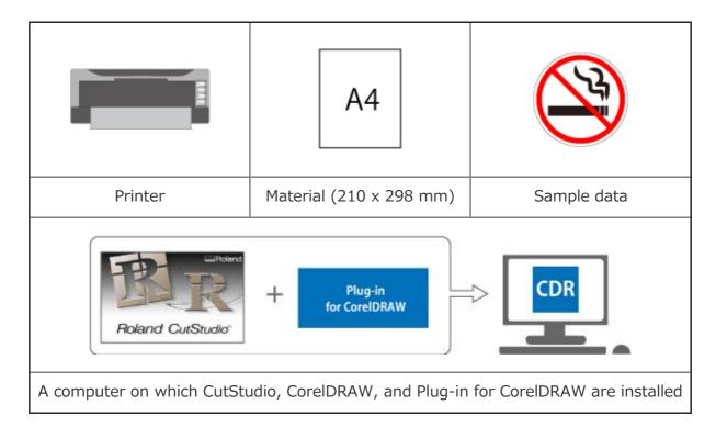
You must use a laser or inkjet printer with a resolution of 720 dpi or greater. If the printed filled sections are blurred, crop marks will not be read correctly.
