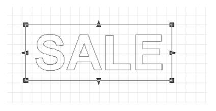
A waste removal line is added around the characters. The character or shape to which the waste removal line has been added is grouped together with the waste removal line. For details on waste removal lines, see the CutStudio help.
