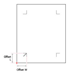
If you want to further reduce the misalignment after seeing the result of printing and cutting, measure the amount of cutting line misalignment, and then add this measured value to or subtract this measured value from the offset values. Set the values as required.
