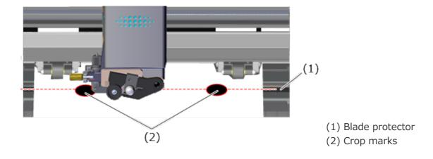
**9.** Press [◀] and [▶] to position the tip of the blade over the center of the lower-left crop mark.
