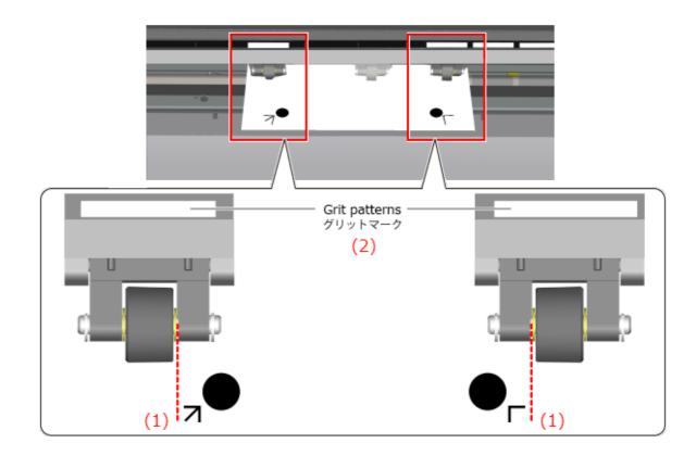
**5.** Align the right edge of the material with the front and back gradations of the platen.
