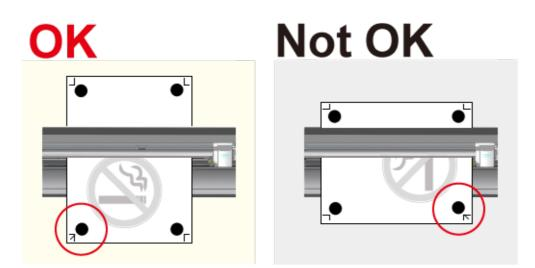
**4.** Position the left and right pinch rollers as shown in the figure.
