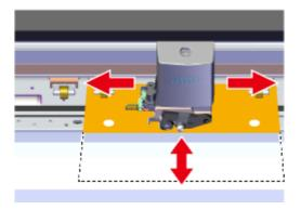
**3.** Align the center of the blade with the position you wish to make the origin.
