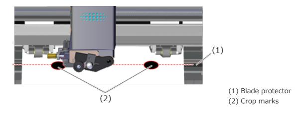
**9.** Press [◀] and [▶] to position the tip of the blade over the center of the lower-left crop mark.
