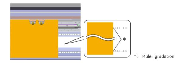
7. Place the left and right pinch rollers over the grit rollers on both edges of the roll material and the middle pinch rollers over their corresponding grit rollers.
