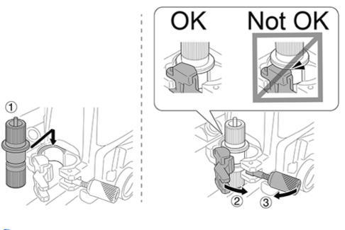
Installing the Cutting Tool
