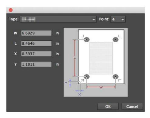
\* When using material with a large amount of feed (long material), we recommend that you set the left and right margins to approximately 25 mm.
