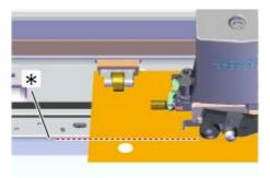
\*: Groove along which the separating knife passes
