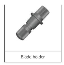
After the tip of the blade has been adjusted, the cap of the blade holder rubs against the material when cutting, causing the end of the cap to gradually wear away. As the cap becomes increasingly worn it becomes impossible to adjust the tip of the blade correctly, and clean cutting is no longer possible. When this happens, replace the blade holder with a new one.
