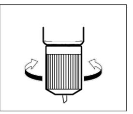
An adjustment of 0.5 millimeters can be made by rotating the cap one full turn.
