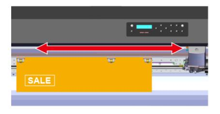
After the material is cut, the cutting carriage returns to the new origin.
