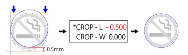
To move the cutting line 0.7 mm up and 0.5 mm to the right  $\rightarrow$  Enter both W and L values
