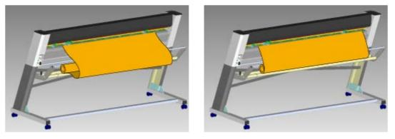
**4.** Place the right edge of the roll material over the grit roller (on the right edge).
