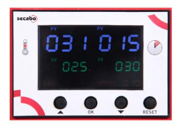
With a large digital controller, temperature (°C und °F) and pressing time can be adjusted. The green digits are showing the theoretical value, the white digits are showing the actual value. A counter (at the right bottom) counts the number of transfers that have already been made since the last reset. The counter can be reset at any time..
