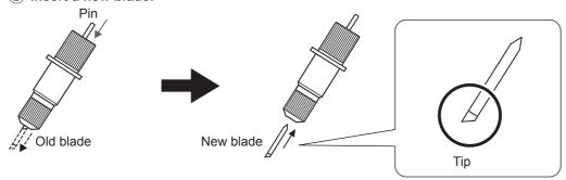
**3** Install the cutting tool in the cutting carriage.
