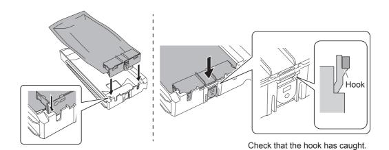
**Set the pouch tray in the cleaning liquid slot.** Insert the ink tray as far as it will go.
