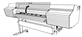
Pass the leading edge of the media between the pinch rollers and the grit rollers.
