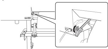
(Move to the front of the printer.) Gently hold down the media and raise the loading lever (front).
