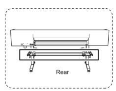
Pass the leading edge of the media between the pinch rollers and the grit rollers.
