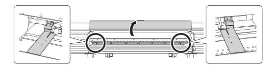
Loosen the retaining screws of the media holders, and then draw them to the left and right ends respectively.
