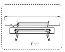
Fit the paper tube (core) of the media on the end cap of the "L" media holder, and then move the "R" media holder to fit its media cap onto the paper tube (core) of the media. Fit the paper tube onto the media holders securely to prevent the media from moving easily.
