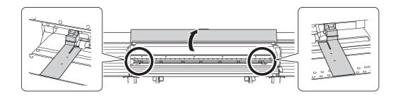
Observe the retaining screws of the media holders, and then draw them to the left and right ends respectively.
