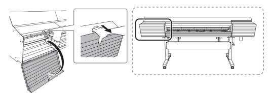
**6** When the following screen is displayed, remove the cut rail.
