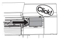
Gently apply pressure from the right side to make sure the print-head carriage does not move to the left.
