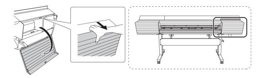
When the following screen is displayed, open the waste valve.
