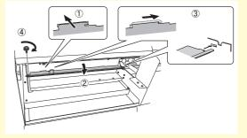
Is the cut rail installed?
