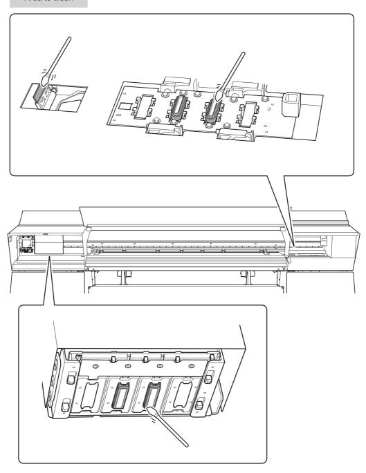
During this work, be careful not to touch the print head surface (nozzle surface) directly with the cleaning stick.
