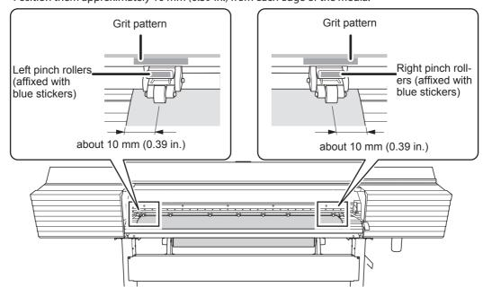
Place the middle pinch rollers over all the remaining grit rollers covered by the media.
