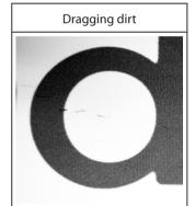
When dirt or dust accumulates on the print head it can interfere with image quality.
